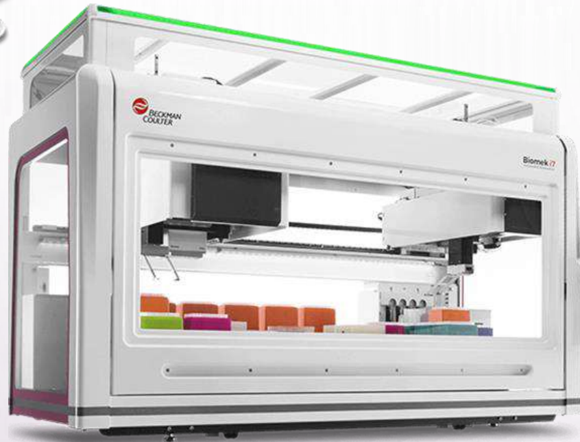
Automatic workstation - Biomek i7 Hybrid (MC + Span-8) with Enclosure
